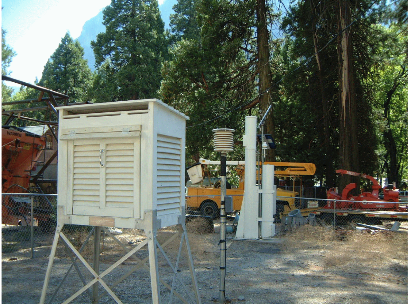
Figure 51. Yosemite Park Headquarters NWS COOP station and MID equipment. Prior temperature sensor locations (Cotton Region Shelter, left; and MMTS “beehive” in center), both NWS equipment, now moved about 140 feet to the left. Third party gauge in rear, precipitation storage gauge (left, with fin), and automated temperature sensor, with satellite transmitter. That station belongs to Merced Irrigation District (MID), and reports via telemetry to CDWR/CDEC in Sacramento. Looking toward south southeast, October 9, 2003. Photo by Kelly Redmond.
