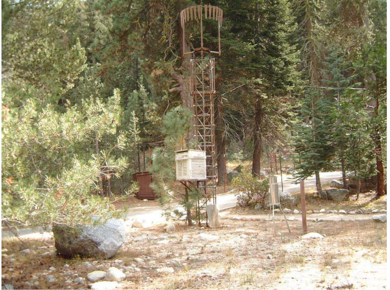
Figure 64. Lodgepole NWS COOP Station view toward southeast showing exposure. Precipitation gauge, Cotton Region Shelter for former liquid-in-glass measurements, tower for since-removed Fisher-Porter recording gauge, looking toward southeast and Lodgepole access road. Photo taken October 11, 2008 by Kelly Redmond.
