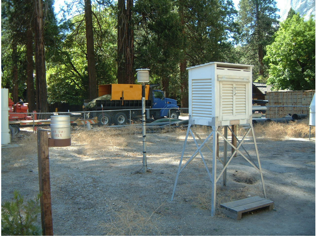
Figure 50. Yosemite Park Headquarters NWS COOP station, old and new thermometers. Previous (right, wooden louvered box) and recent (center, MMTS with radiation shields) temperature sensor locations, and ground surface detail. MMTS system was subsequently moved 140 feet to the left of the viewing angle (in August 2009). Manual US Forest Service precipitation gauge on left (not sure if this is in use). Looking toward southwest, October 9, 2003. Photo by Kelly Redmond.
