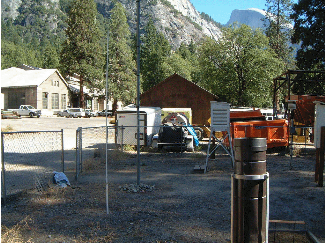
Figure 53. Yosemite Park HQ NWS COOP station and relation to parking and facilities. Observers at this date worked in the dispatch and fire building over the white trailer. Looking toward east northeast, October 9, 2003. Photo by Kelly Redmond.
