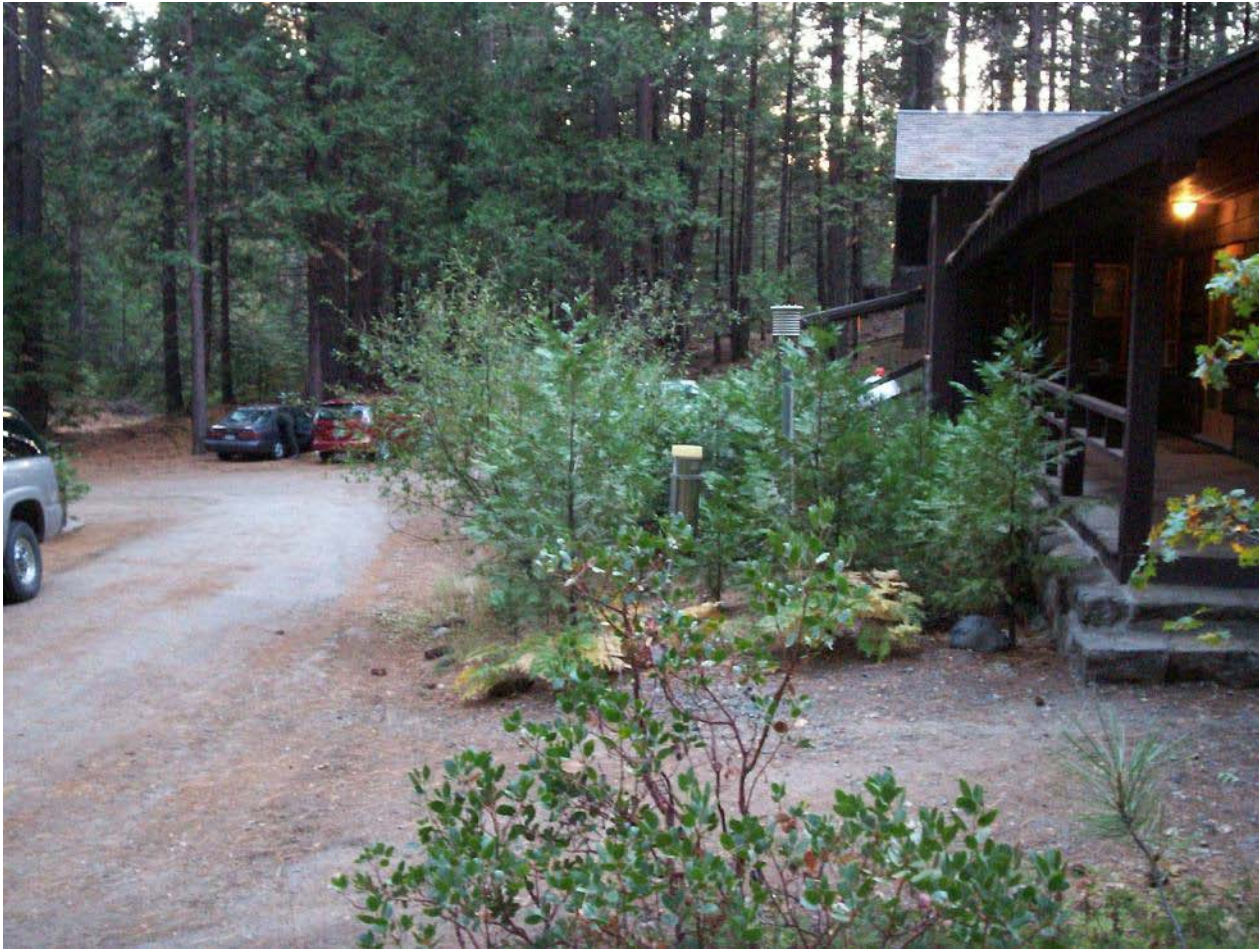
Figure 23. Yosemite south entrance COOP site. With 8" diameter rain gauge (left item in image with yellow funnel top) and maximum/minimum temperature system sensor (MMTS, on taller post). Looking toward west, 2006 October 4. Photo by Kelly Redmond.
