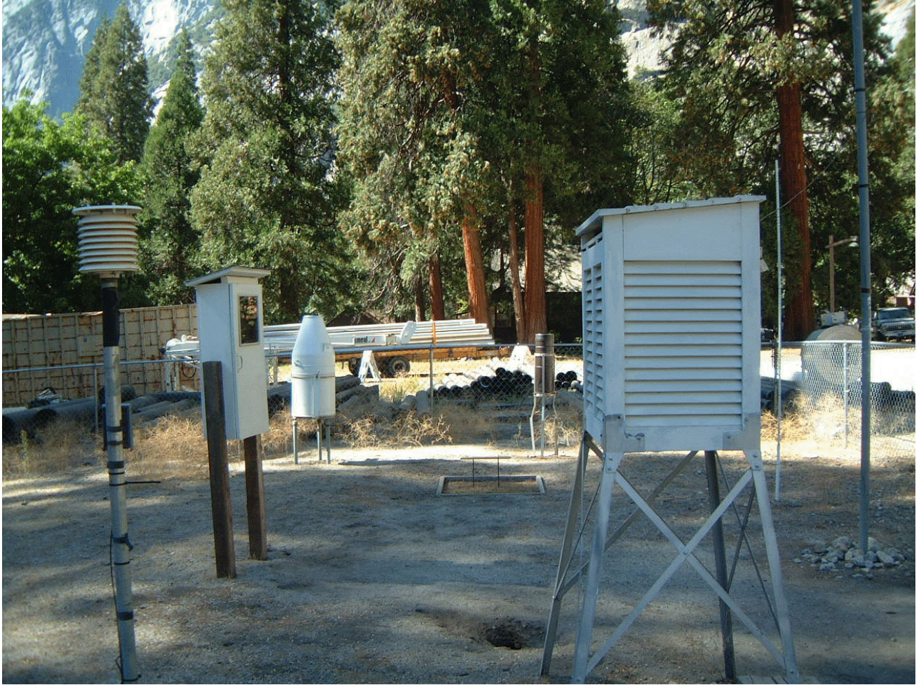
Figure 52. Yosemite Park Headquarters NWS COOP station, toward due west. Foreground: Older Cotton Region Shelter to right, newer style but since-relocated MMTS temperature system to left. Rear: Standard precipitation gauge to right, automated Fisher-Porter precipitation gauge to left. White panel structure to left housed fire weather equipment in the past. October 9, 2003. Photo by Kelly Redmond.
