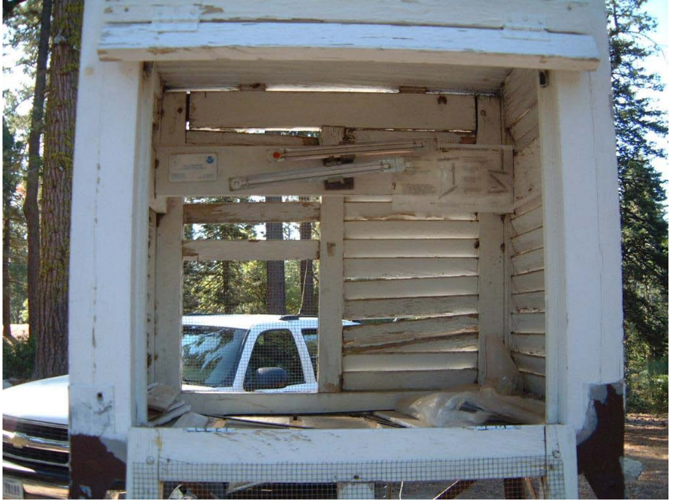
Figure 59. Grant Grove NWS COOP Station Cotton Region Shelter internal detail. Traditional maximum and minimum liquid-in-glass thermometers on Townsend support. Shelter doors always open to due north. Wire mesh has partly replaced louvres. Photo on October 11, 2008 by Kelly Redmond.
