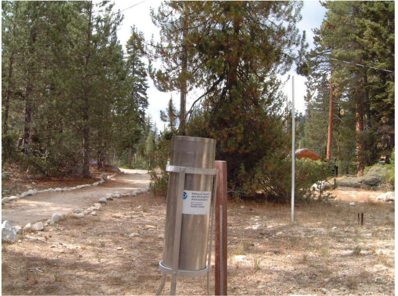
Figure 65. Lodgepole NWS COOP Station hydrology equipment and temperature sensor. Manual 8" Standard Rain Gauge gauge, snow stake for depth to right, MMTS temperature sensor may be the small object extending outward from the peak roof eave of the distant building. Photo taken October 11, 2008 by Kelly Redmond.
