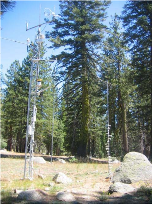
Figure 26. Portion of CDWR Gin Flat automated snow survey site. Shown is portion of the CDWR Gin Flat automated snow survey site, which includes a tower of meteorological instruments. Small tower on right measures temperature every half hour at six inch intervals within snowpack. Photo by Mike Anderson.
