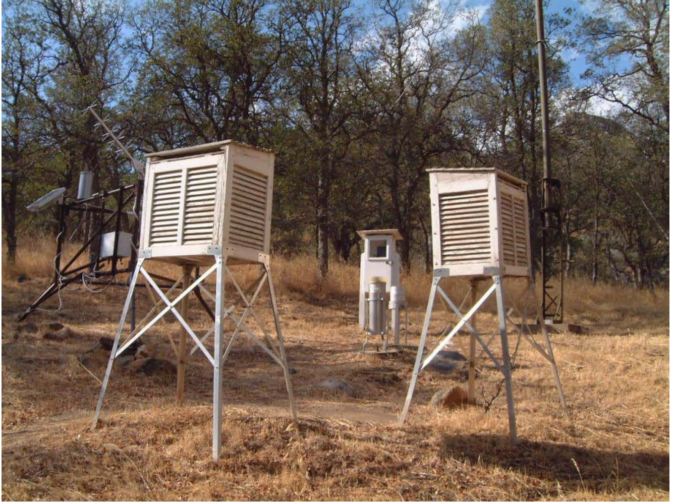
Figure 69. Ash Mountain NWS COOP station, looking toward northeast. Two Cotton Region Shelters foreground, Fire Weather shelter in between, taller NWS Standard Rain Gauge and shorter Forestry gauge, RAWS structure to left, RAWS wind mast to right. Photo October 11, 2008 by Kelly Redmond.
