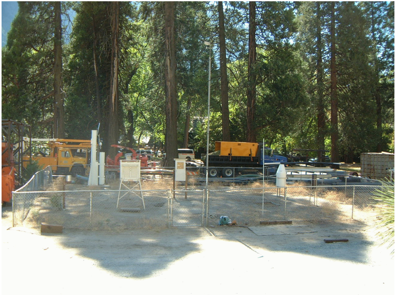
Figure 47. Yosemite Park Headquarters NWS COOP Station, looking toward south. Of interest, from right: Standard 8-inch NWS precipitation gauge (dark cylinder at right), Fisher-Porter hourly precipitation recording gauge (white tapered top), Cotton Region Shelter that formerly housed liquid-in-glass max/min thermometers (atop aluminum cross-braced stand, now unused), MMTS (Max/Min Temperature System behind Cotton Region Shelter, later moved 140 feet to the left), non-NWS equipment for precipitation event reporting (ETI (the manufacturer) precipitation gauge, a CDEC station, owned by Merced Irrigation District (MID, tall white tubes left rear portion of fenced area). October 9, 2003. Photo by Kelly Redmond.
