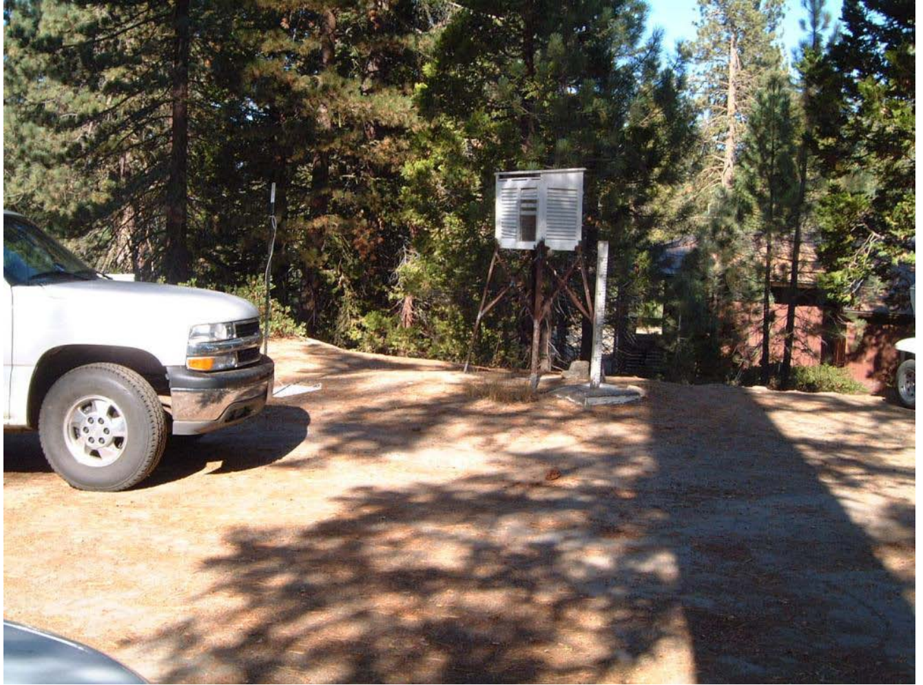
Figure 57. Grant Grove NWS COOP station looking toward northwest and visitor center. Thermometer is in Cotton Region Shelter, snow board in foreground (for daily snowfall), and relation of site to visitor center in right background. Photo on October 11, 2008 by Kelly Redmond.
