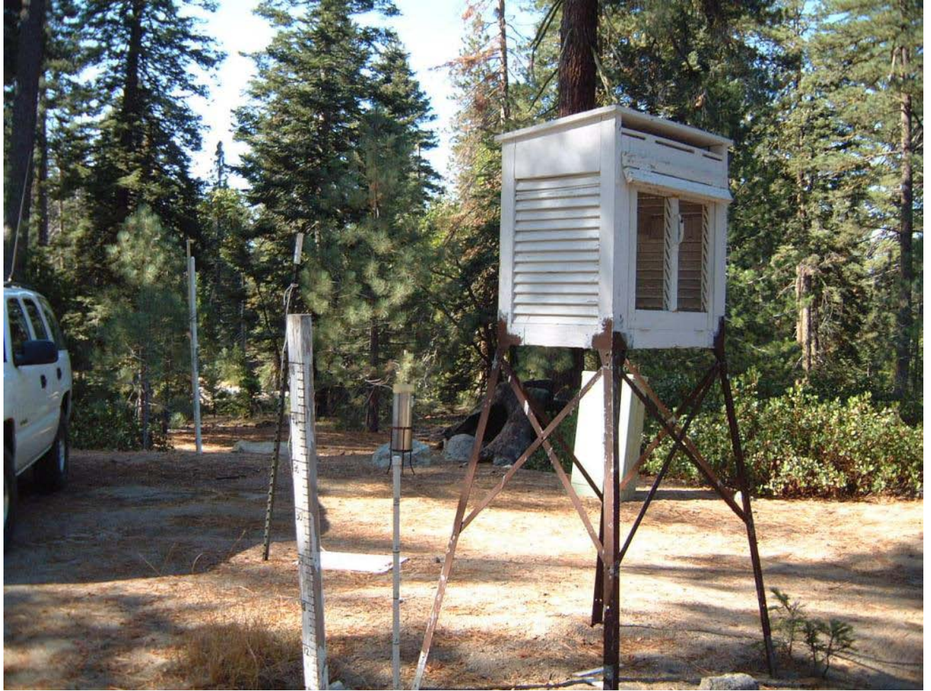
Figure 58. Grant Grove NWS COOP station looking toward southwest with hydro equipment. Relationship of temperature equipment to precipitation measurements: Thermometer is in Cotton Region Shelter, 8" Standard Rain Gauge to left in background, snow board next left (for daily snowfall), and snow stake (for snow depth) next to truck. Photo on October 11, 2008 by Kelly Redmond.
