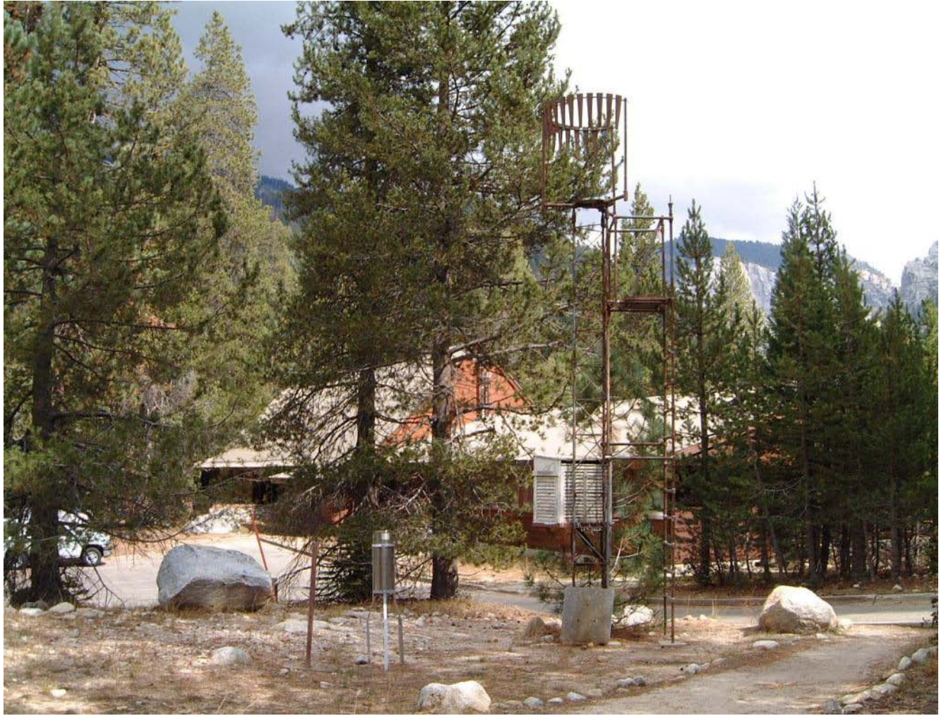
Figure 63. Lodgepole NWS COOP Station at Visitor Center. Precipitation gauge, Cotton Region Shelter for former liquid-in-glass measurements (mounted on ratchets), tower for since-removed Fisher-Porter recording gauge, looking toward northeast toward visitor center. Photo taken October 11, 2008 by Kelly Redmond.
