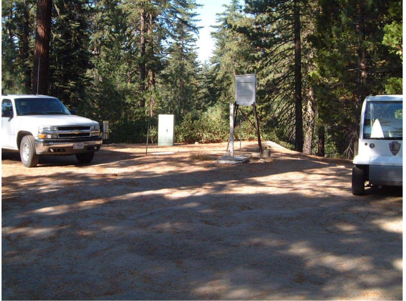
Figure 56. Grant Grove NWS COOP station looking toward due west. Thermometer is in Cotton Region Shelter, snow board in foreground (for daily snowfall), 8" US Standard Rain Gauge behind truck bumper. Photo on October 11, 2008 by Kelly Redmond.
