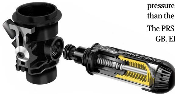
Precisely regulate outlet pressure at the valve regardless of incoming pressure fluctuations with Rain Bird's new PRS-Dial Pressure Regulating Module. This rugged tool optimizes performance by automatically maintaining a constant outlet pressure between 15 and 100 psi (1,0 and 6,9 bars) with an accuracy of plus or minus 3 psi (0,1 bar). Improvements in the design allow precise fine-tuning in increments as small as 1/2 psi.
