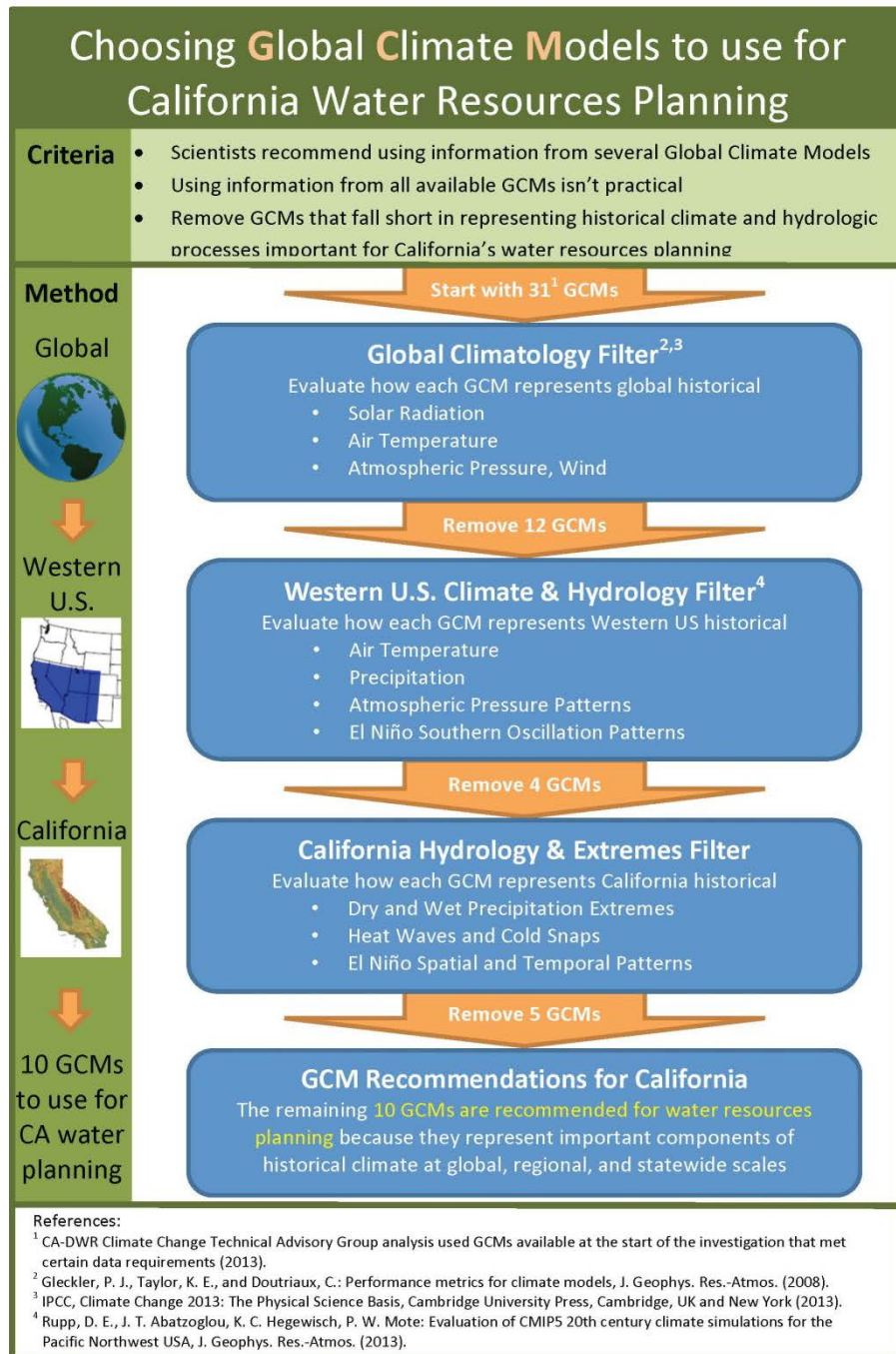
Figure 2-1 Three-Step Process for Selecting Global Climate Models to Use for California Water Resources
